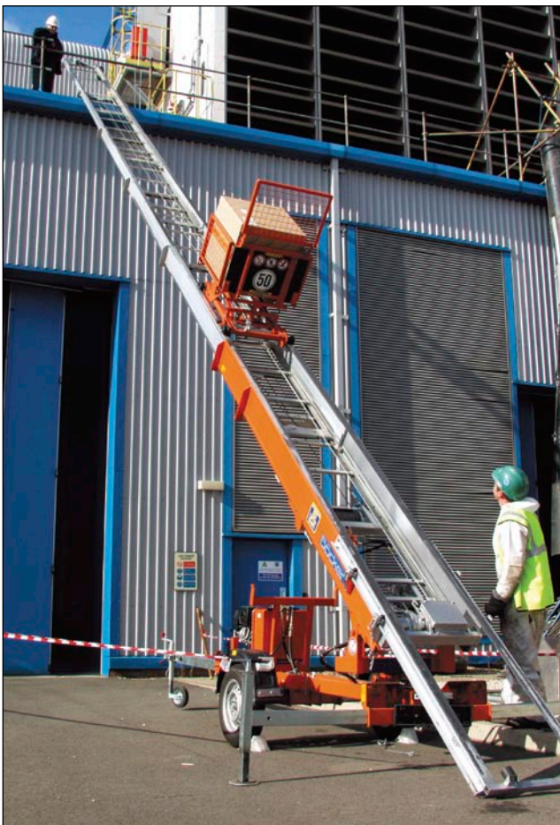
Figure 5(a) Industrial hoist (Images courtesy of HSS)
