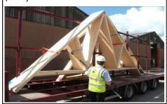
5. The driver will safely mount the vehicle and fit a small ratchet strap around the truss pack and trailer bar at one end only. The driver will then repeat this process to the other end of the pack.
